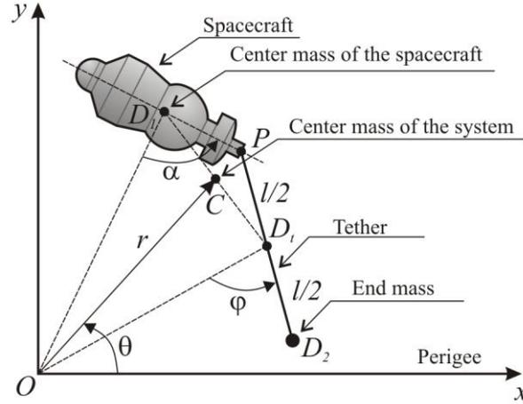
FIGURE 1. Geometry of the tethered system.
